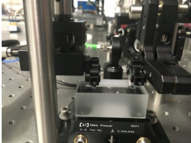
Figure 3.1: Jig Setup for Linear Monolithic Cavity 1
