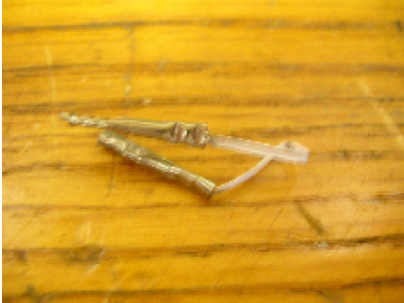
Old thorium-coated electron gun filament.
