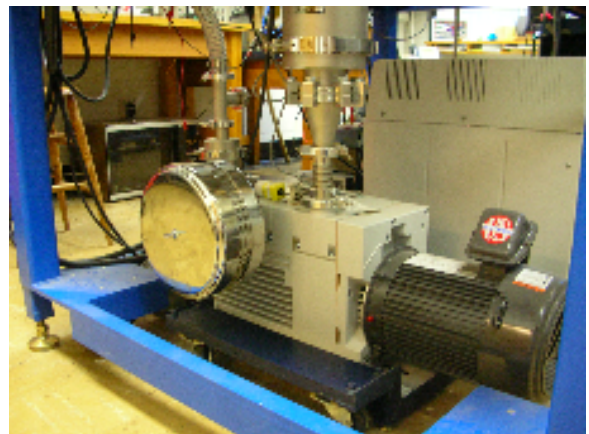
Oerlikon Leybold rotary vane roughing pump with smoke eliminator.
