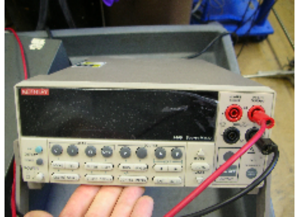
Keithley source meter, set up to measure current from a voltage source.
