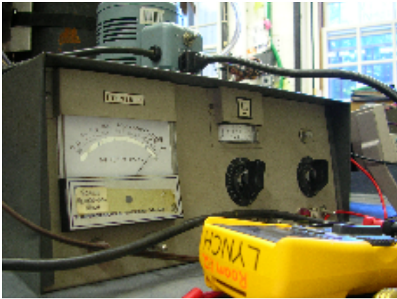
Regular Source Meter used in chamber to apply accelerator voltage and accept ground from the Ketihley.
