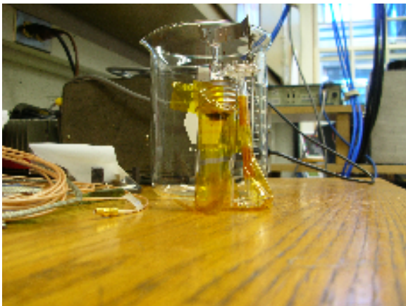
Homemade electron gun using the tungsten filament from an incandescent light bulb.
