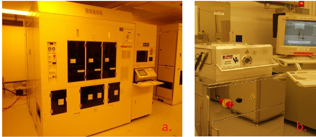
Figure 4.3: NIKON 8 I-liner Stepper (a.) and RIE Unaxis 790 (b.) in the clean room of the University of Wisconsin Madison used in the photo lithography process.
