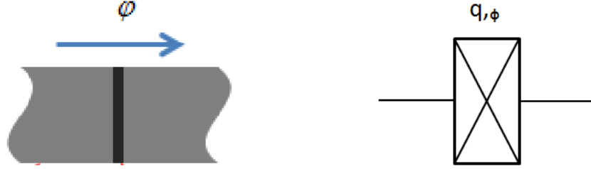
Figure 3.2: Sketch of a single Josephson junction (JJ)
