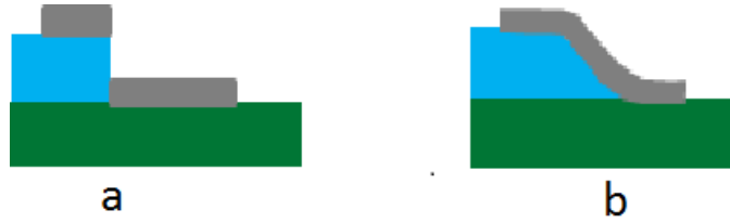
Figure 4.4: Illustration of the effect of having a sloped side wall during Nb etching.
