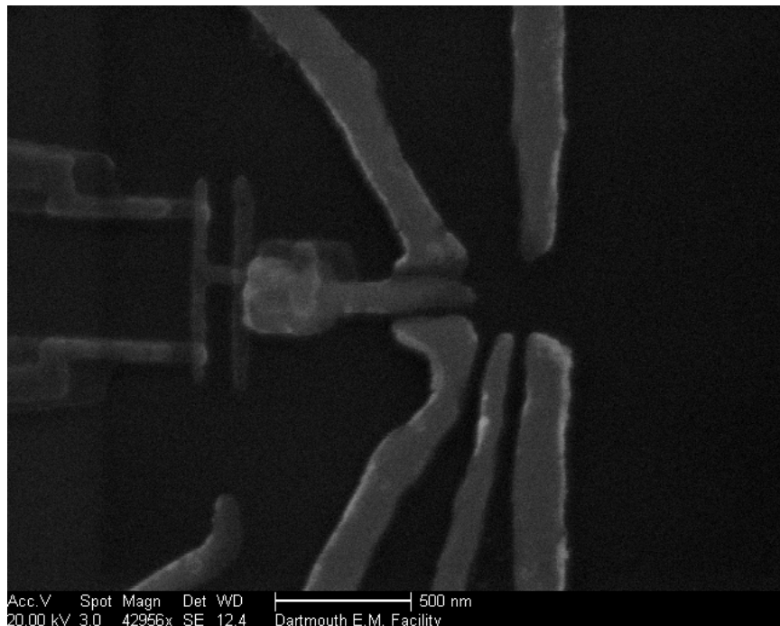
Figure 6.9 SEM micrograph of a combined SET/QD device on Si/SiGe. This is a picture of the actual device that exhibited Coulomb blockade oscillations in the dot. In spite of appearing intact, the SET measured as an open-circuit.
